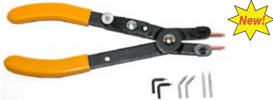
Dual action Snap Ring Pliers quickly converts to install both internal and external snap rings. Includes a set of 4 tips: .045" straight, .060" straight, .045" at 45 degrees, .035" at 90 degrees.
